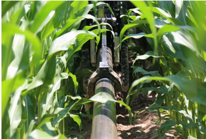
The vertical hose reel uses advanced sensor systems to lay hose as it moves along a backbone path away from the well or hydrant and then picks up the hose as it moves back toward the water source.
