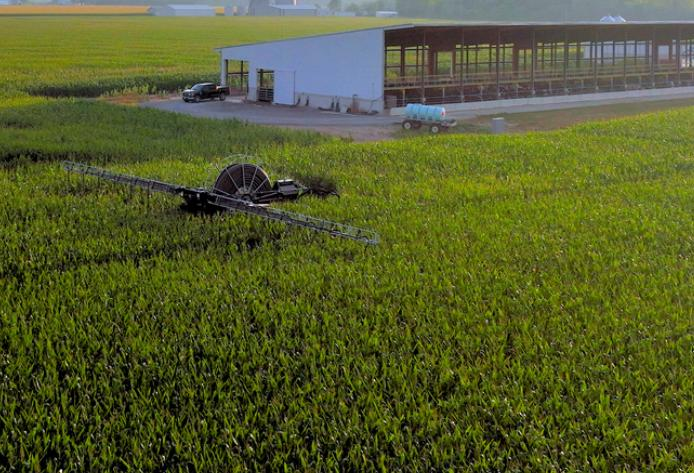
360 RAIN units equipped for manure application include a manure manifold and bucket with an impeller. The impeller breaks up solids and is the final step in eliminating solids and foreign material just before the stream enters the boom distribution lines, eliminating most plugging. Additional screening may still be recommended.
